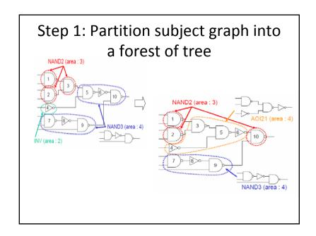
If the gate output has a fan-out of more than 1, disconnect only the output pin from the net. (in tree decomposition, all pins were disconnected)
