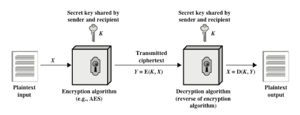
Figure 2.1 Simplified Model of Symmetric Encryption
