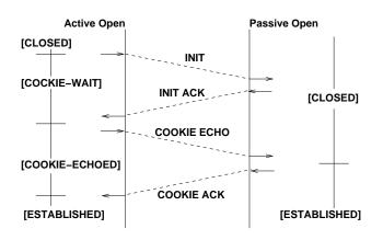
A TCB is not allocated on the server side before the COOKIE-ECHO has been received to avoid TCP's SYN-flooding problem
