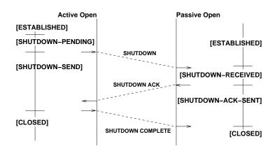
SCTP supports only a full teardown procedure (TCP's half closed connections do not exist in SCTP)
