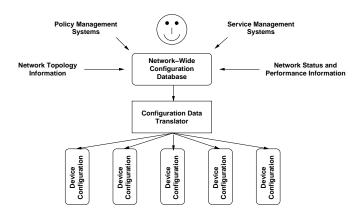
All configuration changes are made (and validated) on the network-wide configuration database and devices are never touched manually
